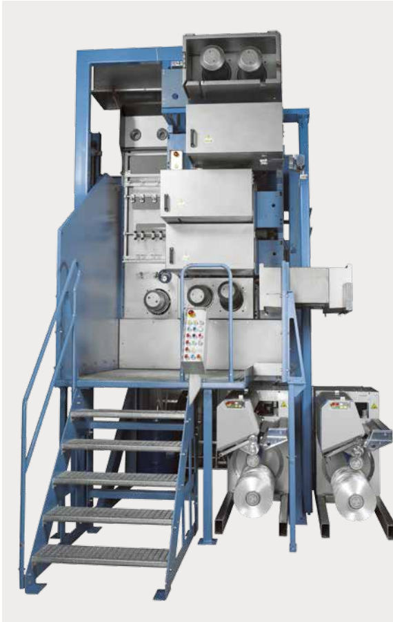
Draw panel with 5 duos for one spinning position
