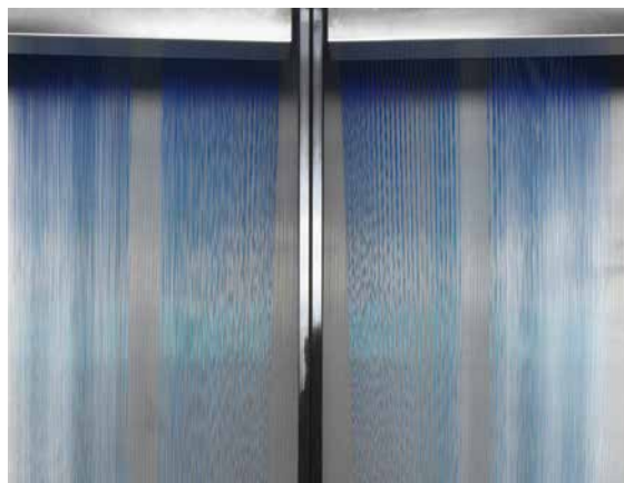
Quenching with 4 end per spinning position
