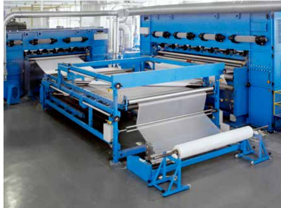
Needling machine installation for filter material
