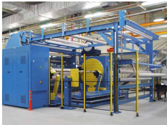
Turret disc winder BWT 202-02 based on Bastian know-how
